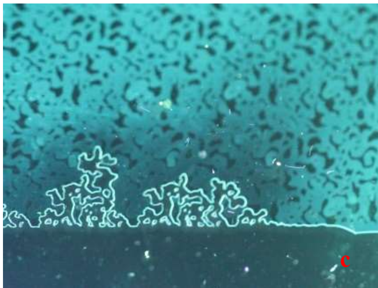
Fig. 2.4—Development of solvent bubbles(heptane and water-wet case): (a) solvent firstly boiled in the fracture; (b) bubbles grew into the pores of the matrix connected with the fracture; (c) bubbles formed a cluster.
