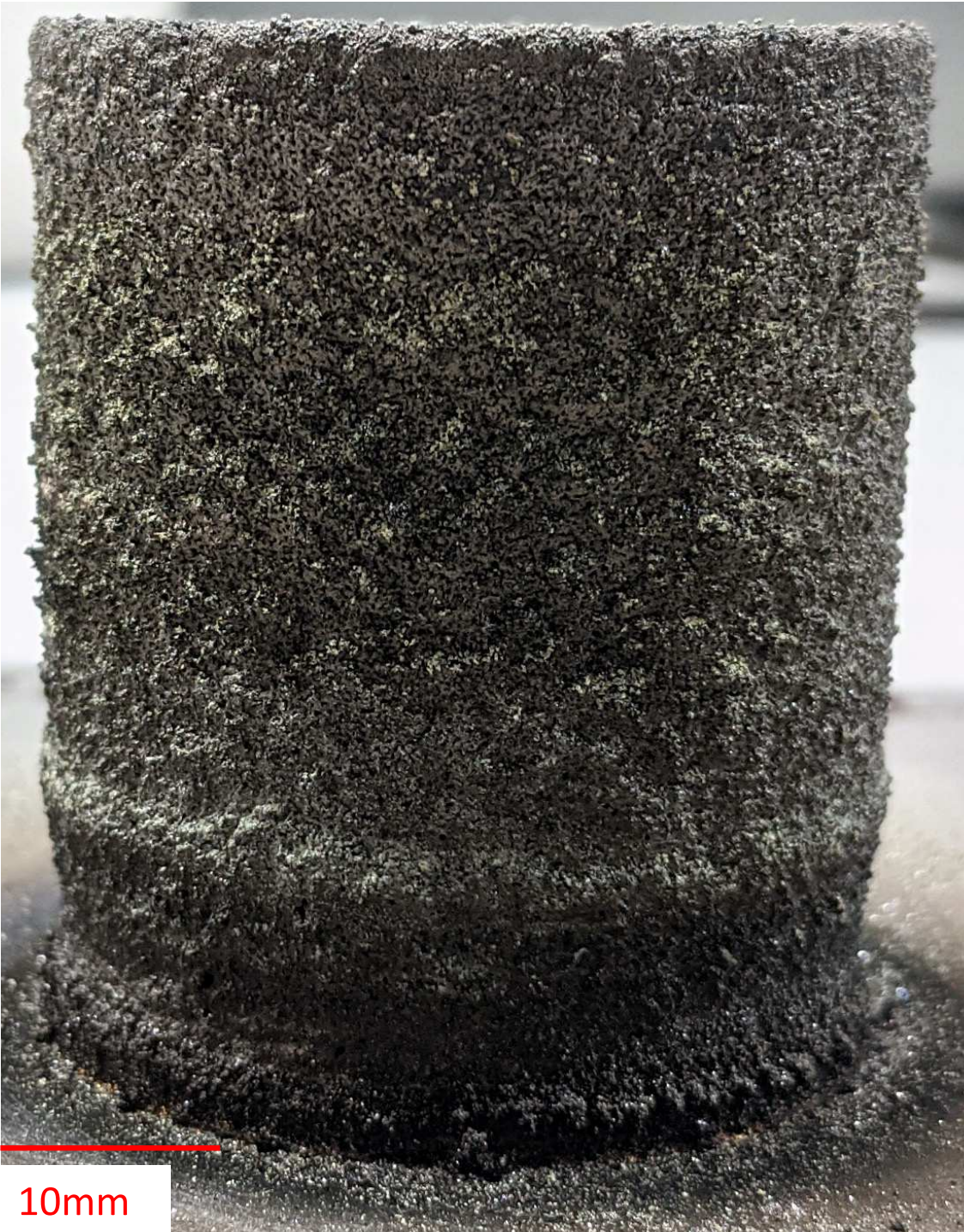
FIGURE 5.6: An example of a PTA-AM build of 70wt% angular monocrystalline WC in a NiBSi matrix. The sample is 50mm tall, and has a diameter of 40mm.
