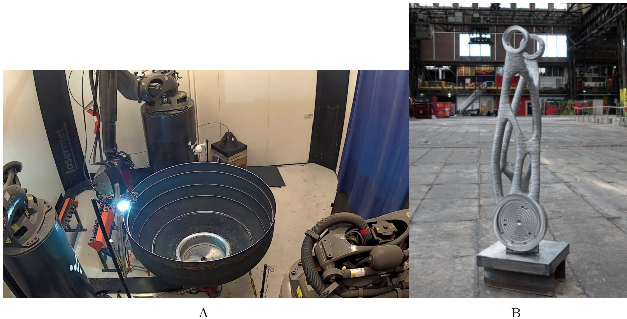
FIGURE 2.2: Examples of companies adopting the large-scale robotic AM technology with (a) a rocket nozzle fabricated by Relativity Space, Inc. [72] and (b) a component of a serial manipulator fabricated by MX3D [73].
