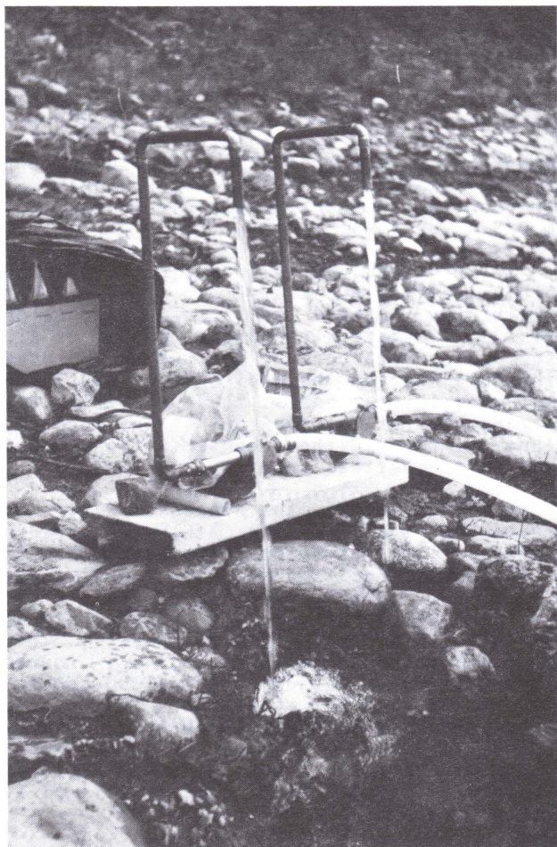
Fig. 1. Pumping apparatus for subsurface water sampling.
