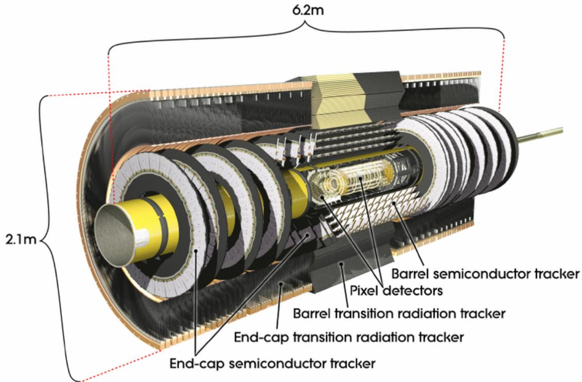
**Figure 4.4:** Cutaway diagram of the ATLAS inner detector [55].
