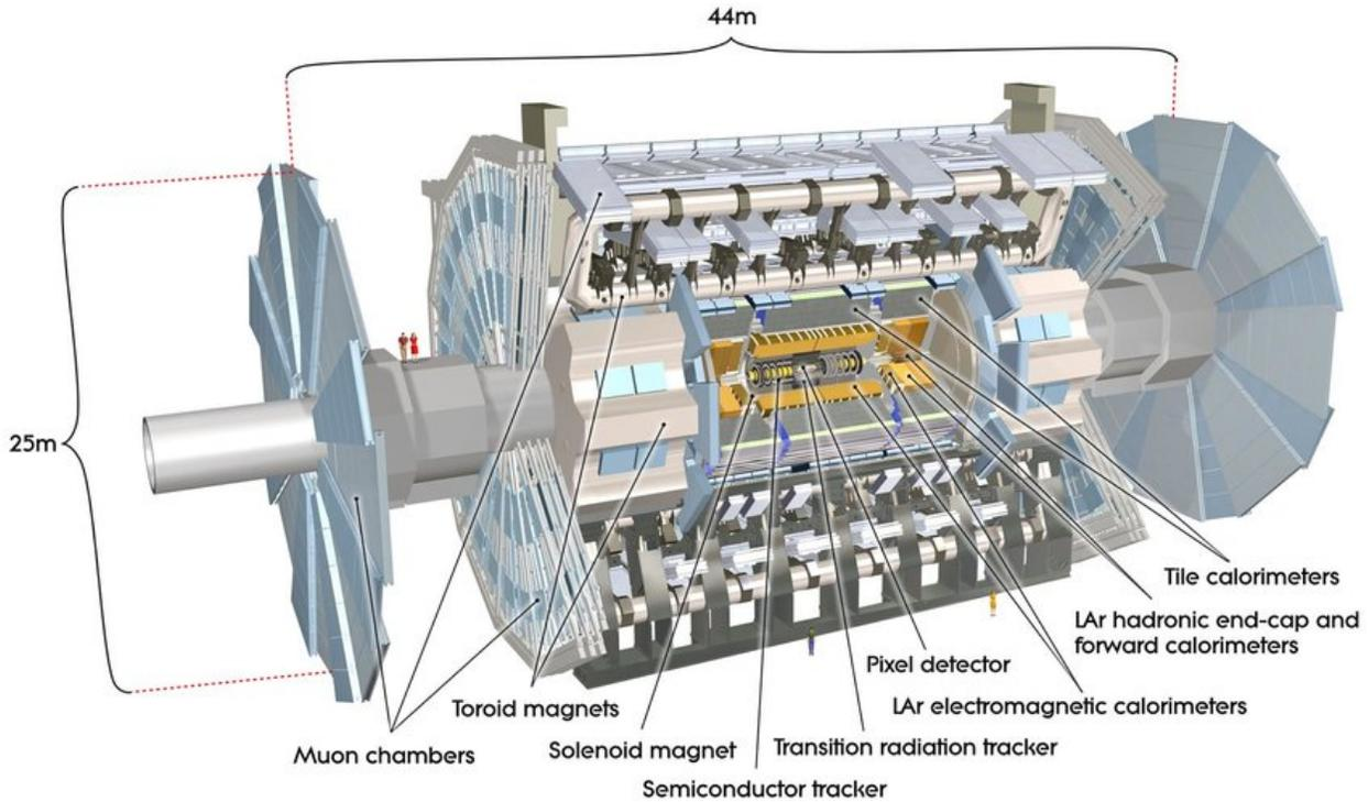
Figure 4.3: Cutaway diagram of the ATLAS detector [55].
