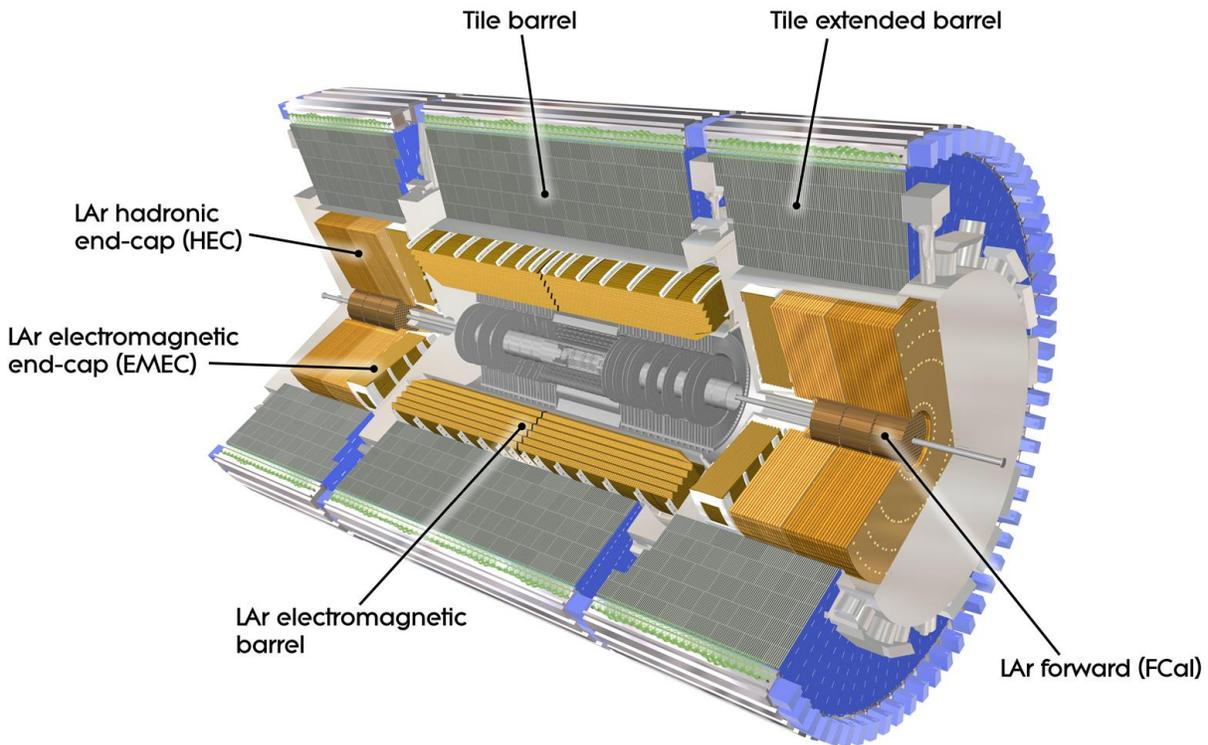
**Figure 4.5:** Cutaway diagram of the ATLAS calorimeter system [55].
