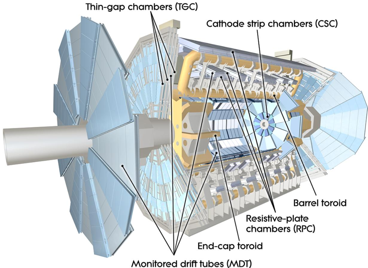
**Figure 4.6:** Cutaway diagram of the ATLAS muon system [55].
