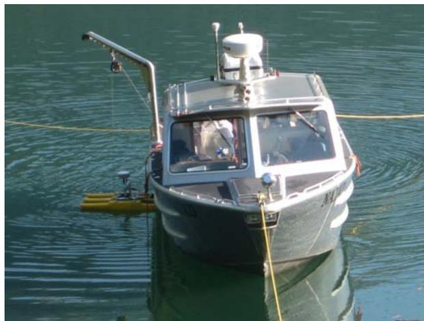
Figure 4.6 Sentinel ADCP measurement set-up: (a) schematic, (b) ADCP in mooring cage on hydraulic winch cable before deployment, and (c) deployed ADCP with RTK measurements from trimaran.
