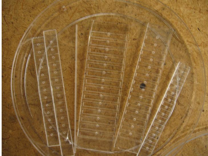
Figure 3.7: A series of waveguides on 4" long substrates were produced using nanofabrication methods
