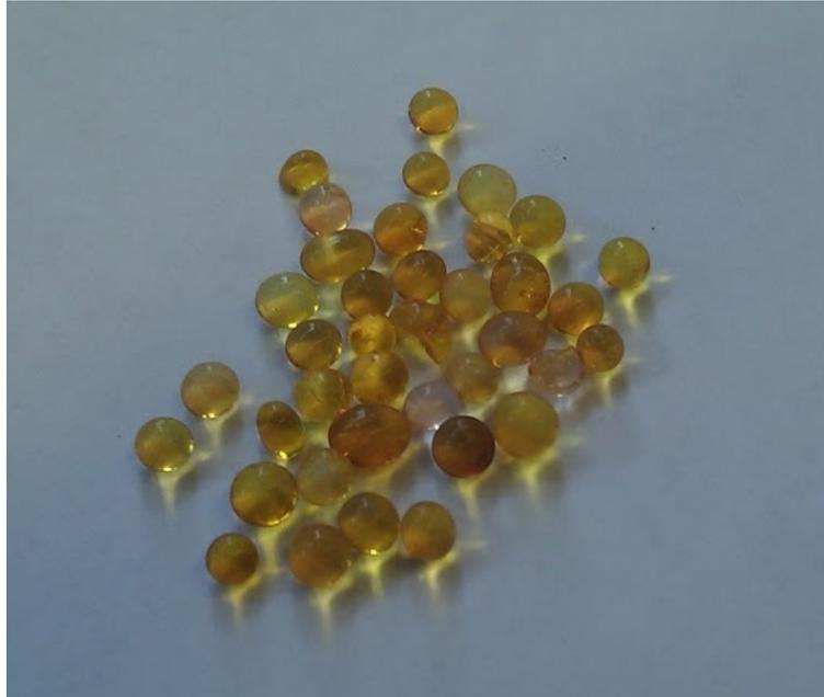
**Figure 2.5:** *Silica gel bead dessicant*
