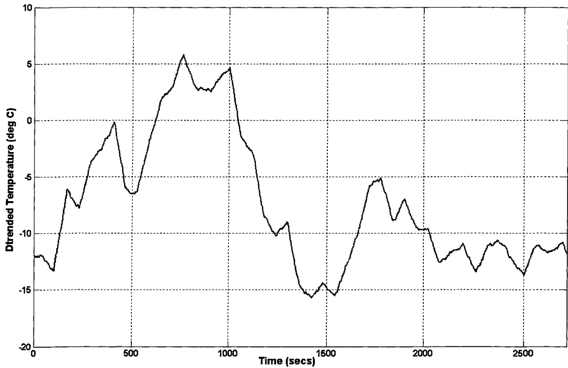
Figure 6.23: Integrated white noise disturbance sent to Heated Tank closed loop.
