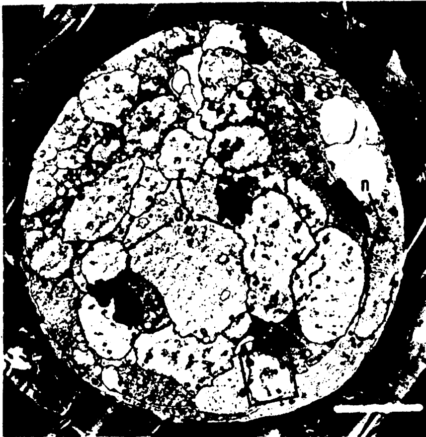
Fig. 2 Thin section through one of the channels remaining after several 25- \mu m strands were etched out of an epoxy wafer; scale mark, 5 \mu m. The section had been fixed in glutaraldehyde, postfixed with osmium tetroxide, and stained with uranyl acetate and lead citrate. Flakes of epoxy torn off by the ultramicrotome obscure small portions of the cross section. Note several irregularly-shaped axons, three of which are indicated by the arrows converging at the marker (ax). Note the nucleus of what appears to be a Schwann cell, marked (n).
