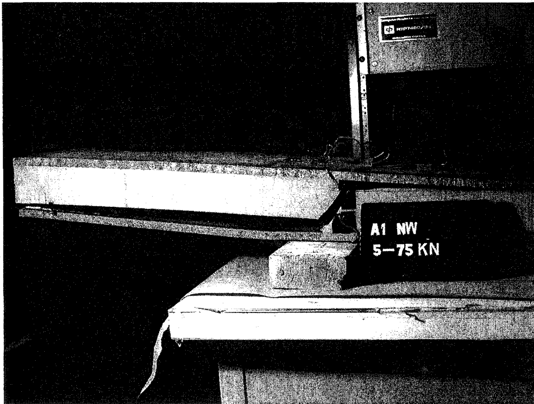
Figure 4.2: Failure of the steel-elastomer interface (A1 shown).
