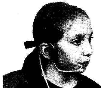
Figure 1.3: The Sip/Puff Switch with Headset (Origin Instruments, Corp., USA) that was used in the study.
