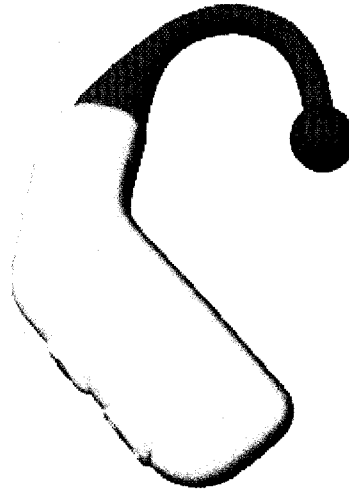
Figure 1.4: Current tooth-click detector prototype showing case (grey) and sensor arm (black) geometry.
