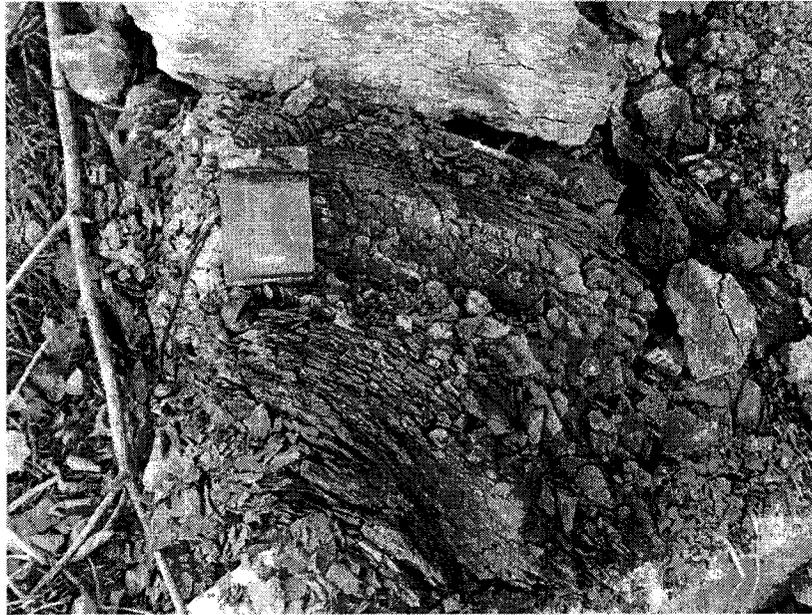
(a) Disintegration of a block of Opalinus Clay.
