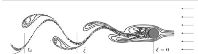
Figure 8.1: Vortex shedding in the 2D flow behind a cylinder [2]
