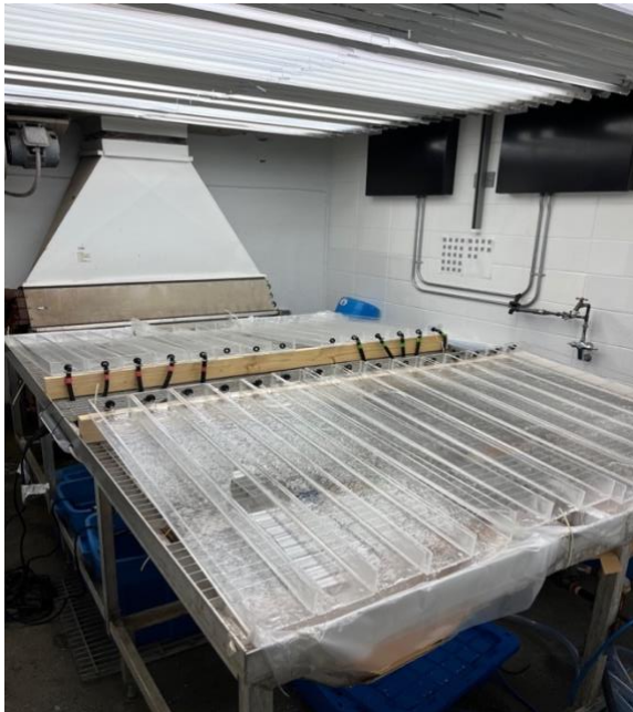
Figure 3.2. Left – Artificial stream mesocosms in a controlled growth chamber at the University of Alberta. Right – Experimental set-up with five unglazed terra cotta tiles colonized by epilithic algae placed into each of 20 stream channels.
