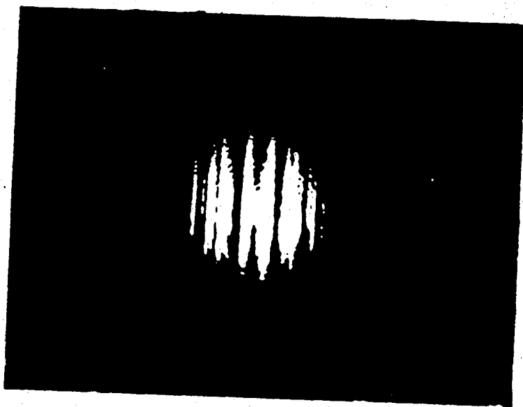
Figure 2-5. Beam profile for the high precision laser-based refractive index determination within picoliter volumes using flow-modulation of the sheath-flow cuvette. (a) When the valve is open, the sample does not interact with the laser beam and an unperturbed beam profile is observed. (b) When the valve is closed, the profile is established, the sample interacts with the laser, and the perturbed profile is observed.
