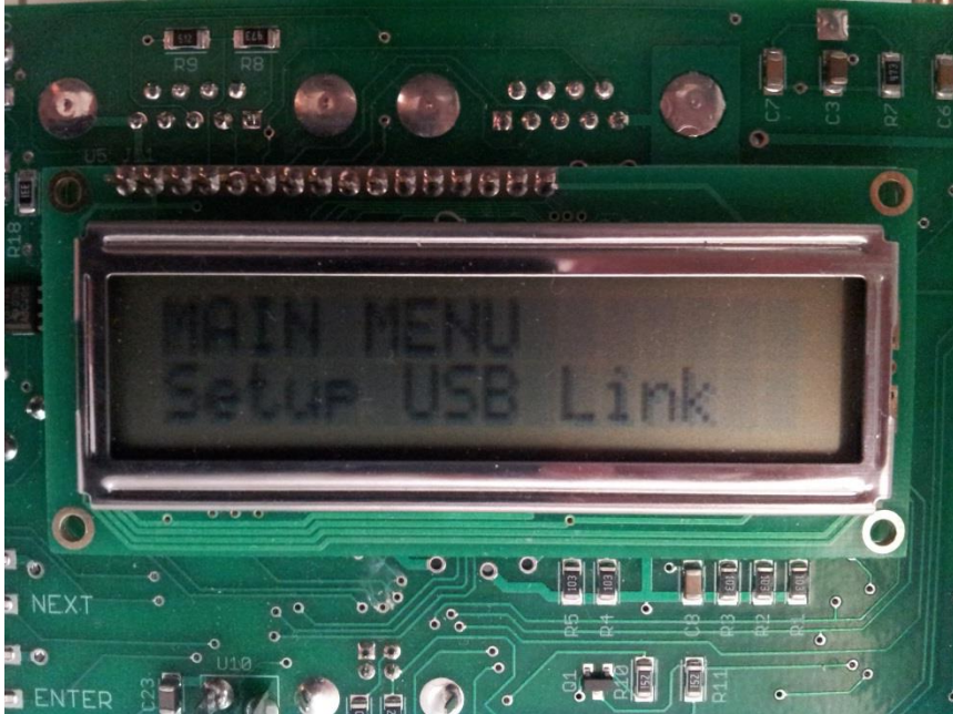
Figure B. Image of the remote advanced playback unit (RAPU) LED display.
