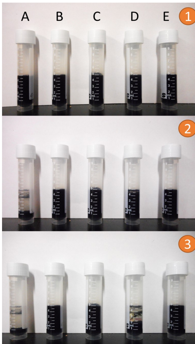
Figure 4.22: Photographs of magnetic filler settling experiments, taken at (1) immediately, (2) 3 hours, and (3) 24 hours after filling the test tubes. (A) 0wt% rheological additive, (B) 0.5wt% BYK 7410 ET, (C) 2wt% BYK7410 ET, (D) 0.5wt% Disparlon 6900-20X, (E) 2wt% Disparlon 6900-20X.
