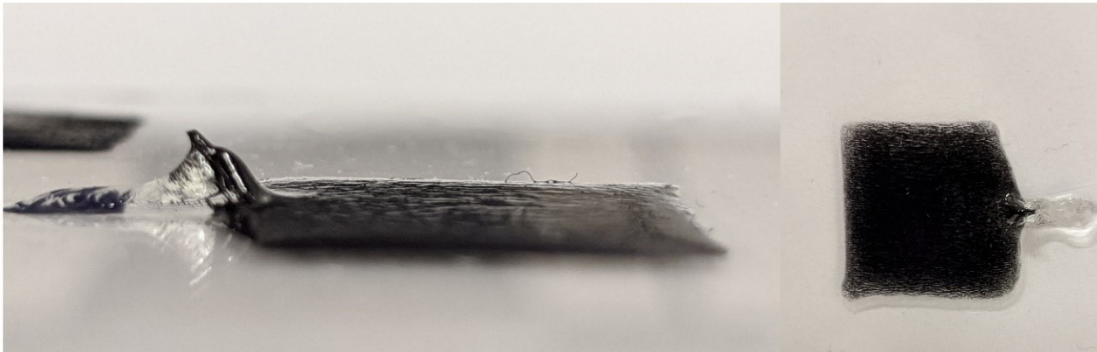
Figure 5.11: 3D printed magnetic composite with observed deformation artefact due to the magnetic field.
