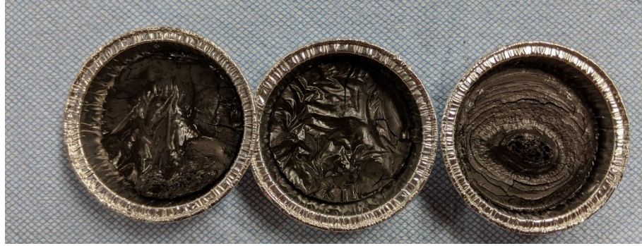
Figure 7.11: Specimen cracking observed at a lower magnetic filler loading
