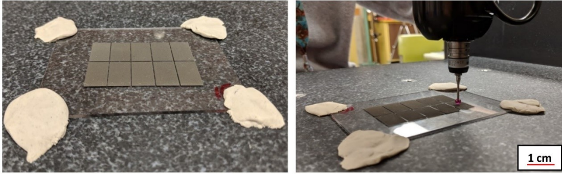
Figure 3.4: Thickness measurement setup for acquiring data for the working curve model: (a) Fixing a sample by securing four corners of the acrylic substrate with plasticine on the CMM granite table; (b) Measuring the thickness of a rectangle of a sample using the CMM probe.
