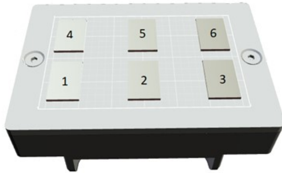
Figure 3.2: Arrangement of samples for dimensional accuracy experiments. Numbers on samples represent printing zones 1 to 6 on the build head.
