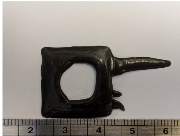
Figure 7.12: Deformations observed with NdFeB formulation materials
