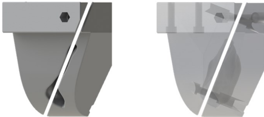
Figure 46. Model of 3D-printed pelvic fixture designed for experiment, showing the part as a solid and with translucency to show the clamping bolt holes and the SI joint conforming profile.
