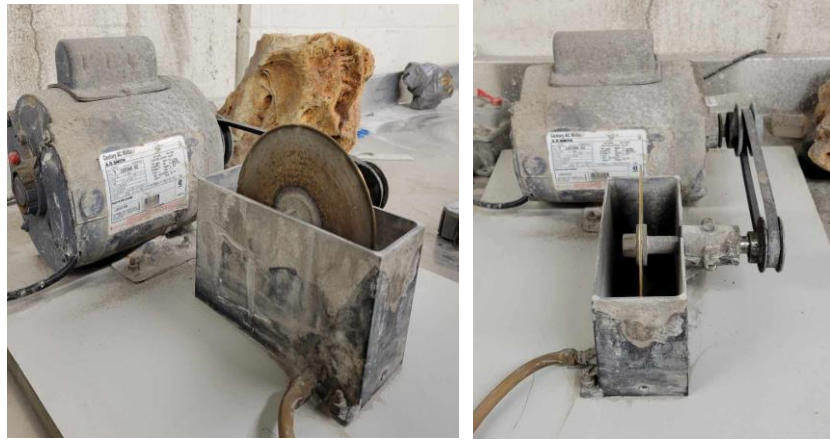
Figure 4-3: Diamond saw used for cutting the cement cores
