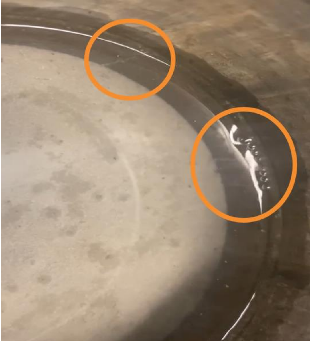
Figure 3-2: Visual inspection to determine the fluid flow pathway across the neat G cement plug with 25% water contamination.
