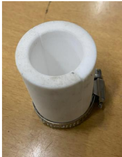
Figure 4-2: PTFE mould used to cure the bulk cement core
