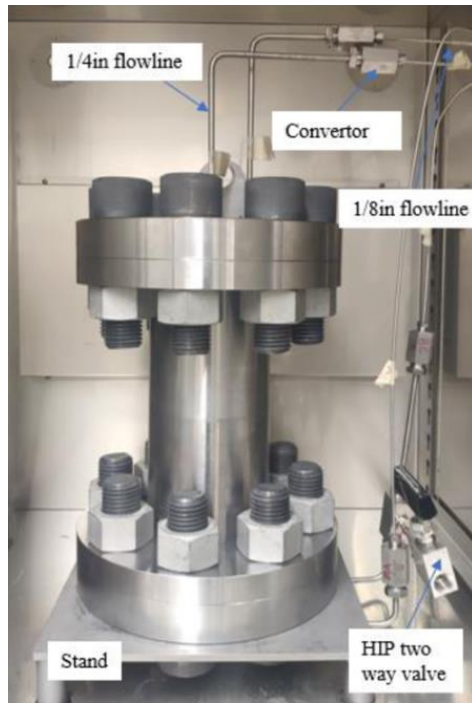
Figure 2-5: Wellbore simulator placed inside an oven [27].
