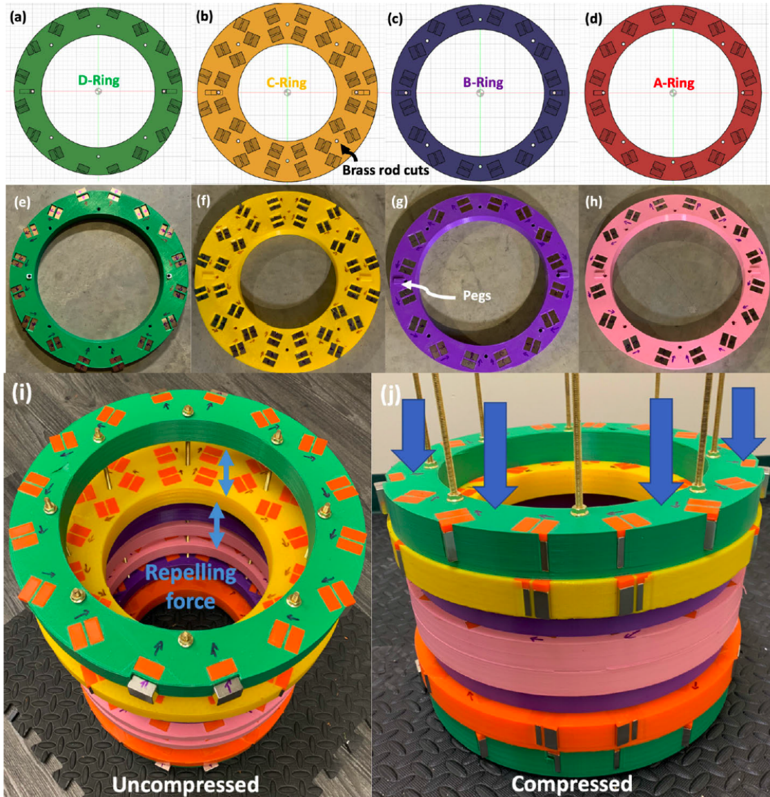
Figure 4.16: Construction and assembly of the Halbach magnet. Photos of the four (out of 8 total) designed (a-d) and manufactured (e-h) formers. The other four rings (not shown) are identical. The 3D printed formers with N40UH magnetic blocks fitted into pockets are shown. Eight cylindrical (6.35 mm diameter) cuts in the CAD models allow throughput for brass rods, and the pegs/holes in formers minimize ring shifting when compressed. (i-j) Flange brass nuts are tightened, compressing the rings (blue arrows) into their optimized geometry.
