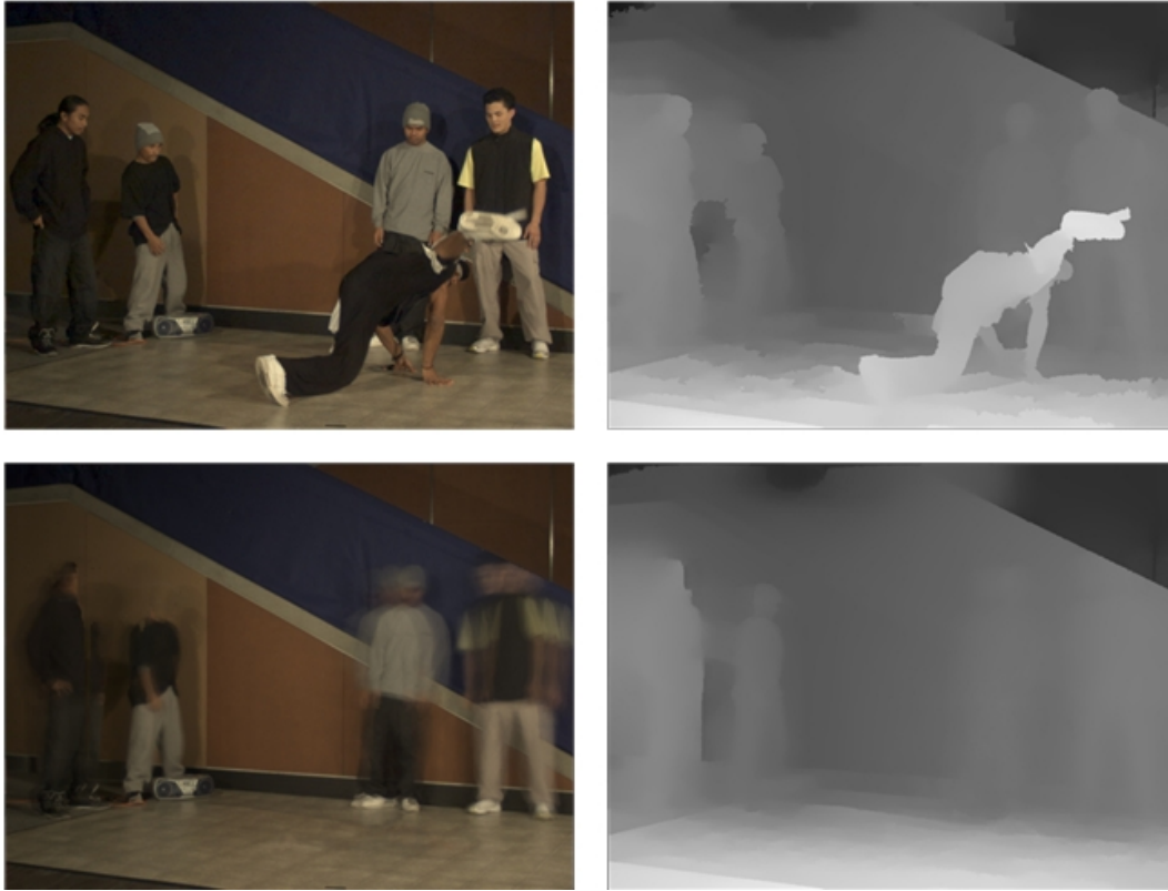
Figure 3.16: Top row: A color image and its corresponding depth map. The view-point is different from the ones in Figure 3.15. Bottom row: Estimated background.
