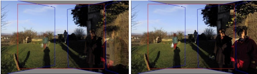
Figure 2.4: Left: Result when applying a typical image stitching system. Right: Result by applying some method for ghost elimination. (from [56])
