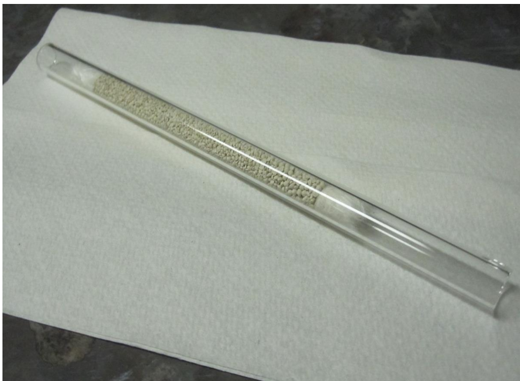
Figure 2-4. Sample adsorbent bed packed with zeolite 4A pellets
