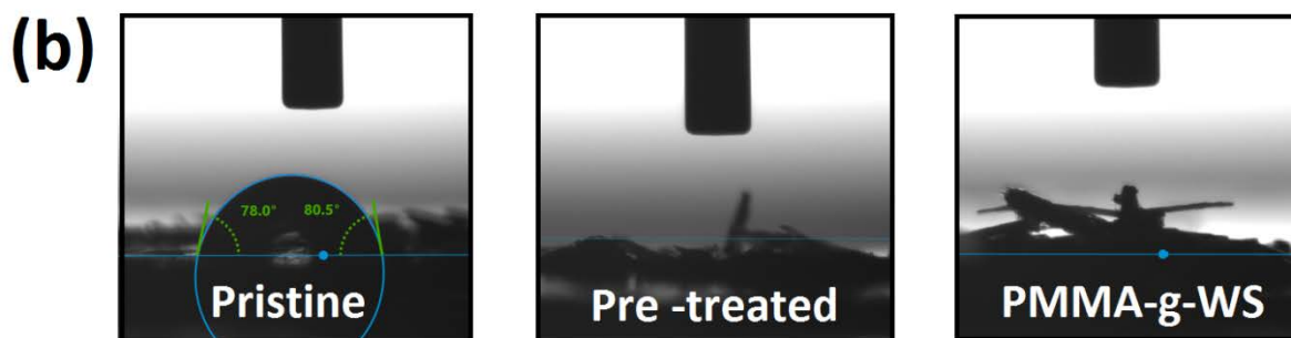
Figure 2.5 Water contact angles of pristine, pre-treated, and PMMA-g-WS in three different time-steps and oil contact angles of all the three adsorbents (b).
