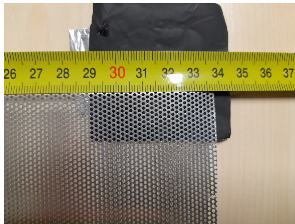
Figure 4.37: A picture of the perforated mesh used, along with a ruler for scale.
