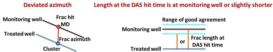
Figure 5.17: Schematic of the expected characteristics displayed in the fracture connection map, and PKN analysis for Scenario 4.
