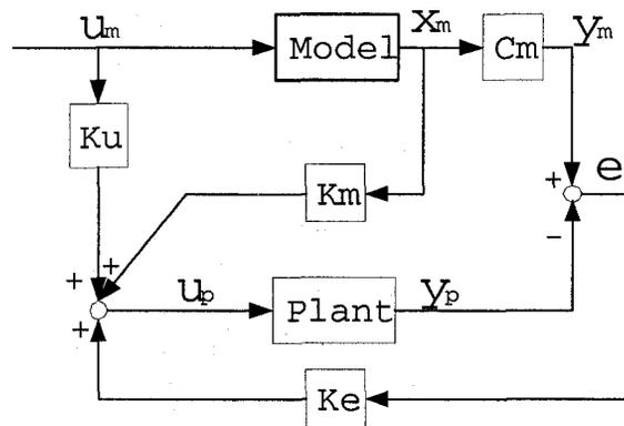
Figure 1.3. Block diagram of explicit model following
