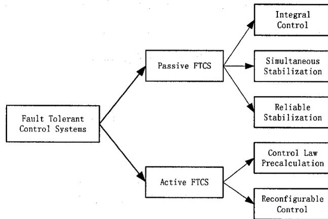
Figure 1.1. A simple classification of fault tolerant control systems
