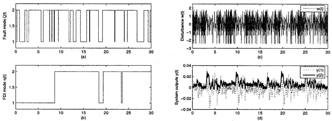
Figure 5.2. Single sample path simulation using the decentralized controllers: (a) fault modes; (b) FDI modes; (c) system disturbance; (d) system outputs.
