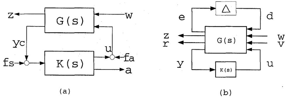
Figure 1.4. Four-parameter controller structure : (a) system setup (b) standard setup with model uncertainty
