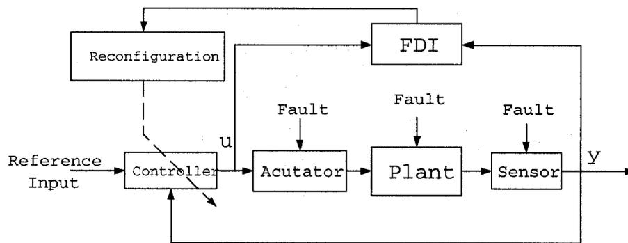
Figure 1.2. A scheme of active fault tolerant control systems
