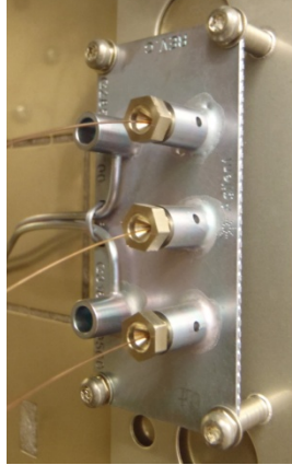
Figure 2-4. Agilent's commercially available Deans switch plate.
