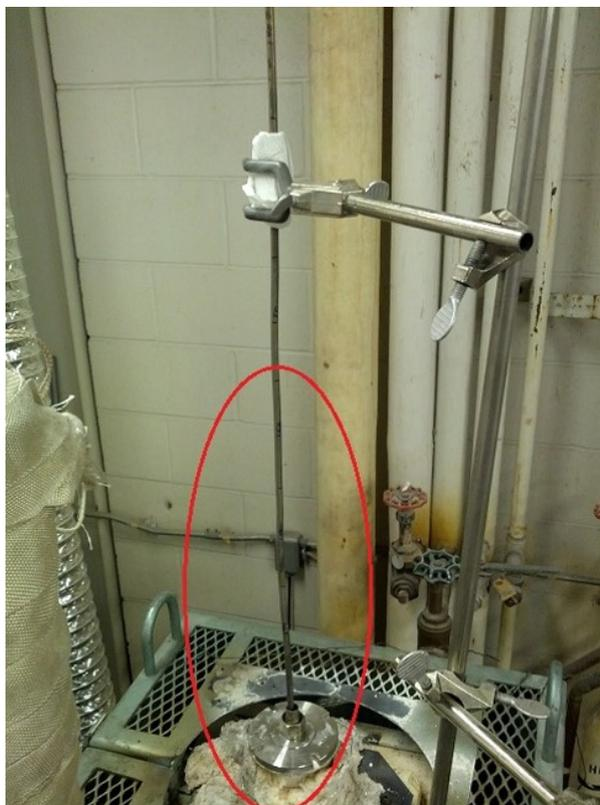
Figure A-5: Experimental setup for calibrating the DTF
