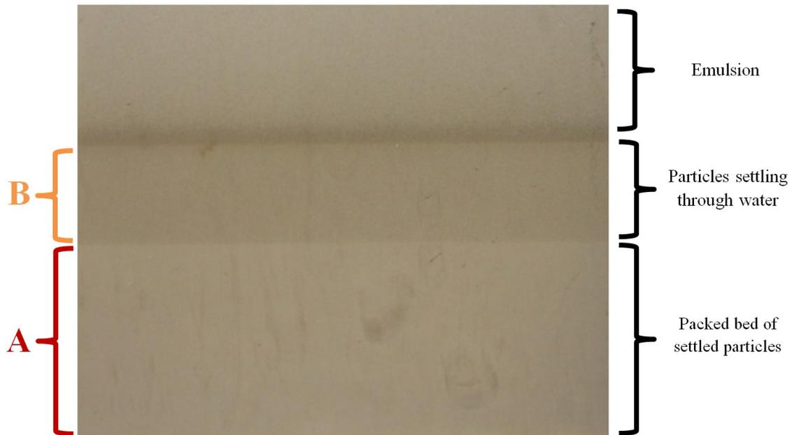
Figure 5.2- The particles after being disengaged from the rising emulsion are divided into two zones: settling particles through water (zone B) and packed bed of settled particles (zone A)
