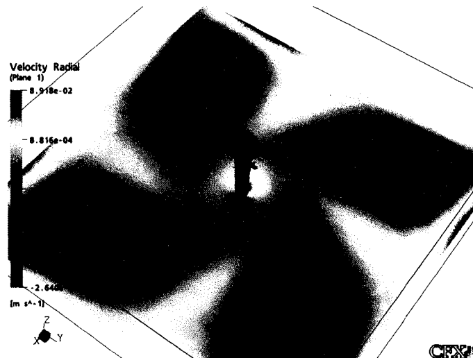
Figure 5.43: Vorticity isosurface in the Open model showing the velocity field at a cross-sectional plane.
