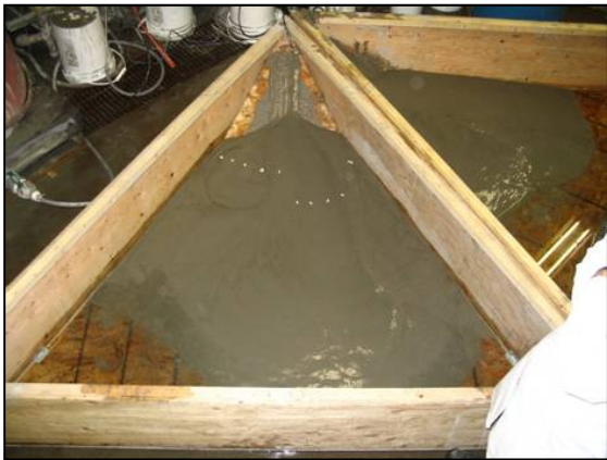
Photo 7. Larger Scale Deposition Test (Modified Flume)
