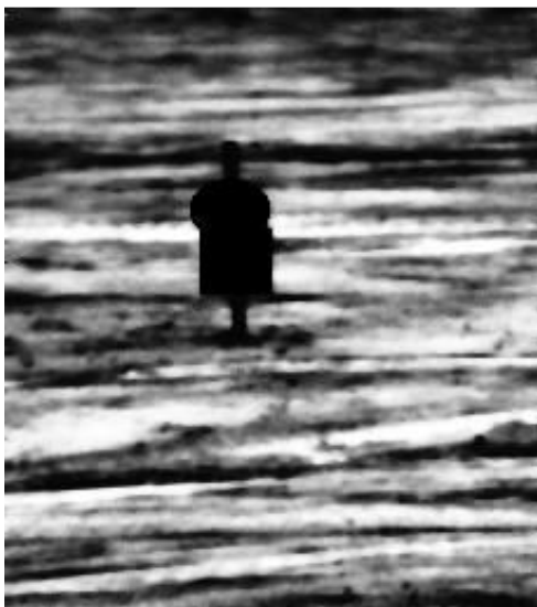
Figure 7. Black & white Hypercam processed image showing the classification of sand-rich regions in brighter tones and fines-rich regions in darker tones.
