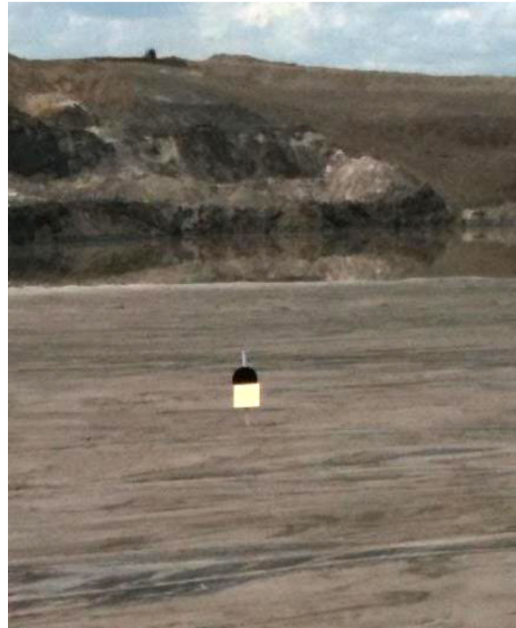
Figure 6: Visible image of a coarse tailings deposit, with gold square and circular black calibration panels shown in the centre of the image, and released water and pit wall shown in the background.
