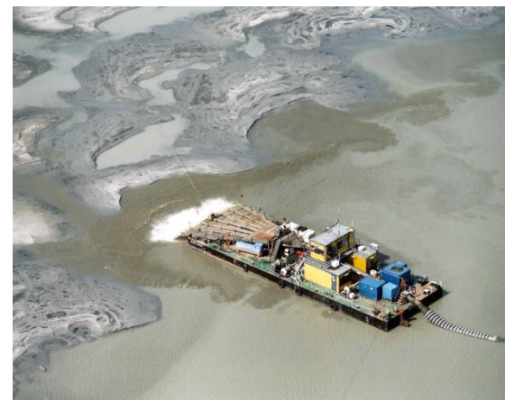
Figure 8. Large scale production surface diffuser (complements of Van Oord) with rainbowing above and raining by surface diffuser below.
