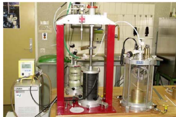
Figure 3. Seepage Induced Consolidation (SIC) test apparatus.
