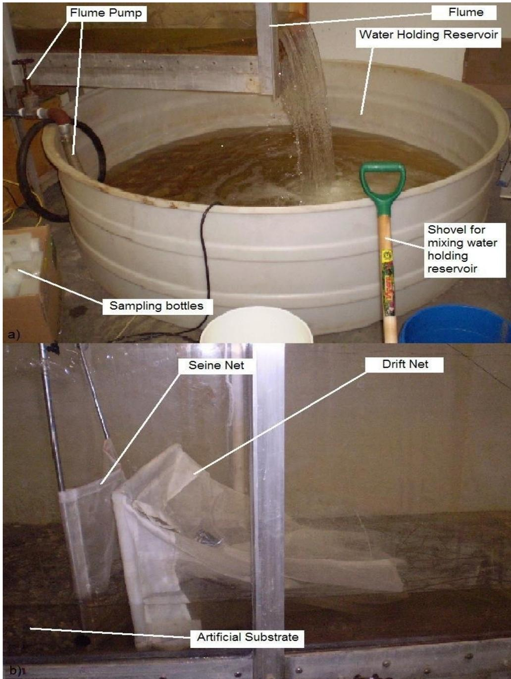
FIGURE 3-3 a) Close-up of the water holding reservoir, showing water entering from the flume and being pumped out by the flume pump. During the experiment sodium sulphite was added to the water holding reservoir and the water holding reservoir was mixed with a shovel; b) Close-up of the configuration of the seine net and drift net downstream of the artificial substrate, where the seine net blocks the entrance of the drift net when the experimental run is not occurring
