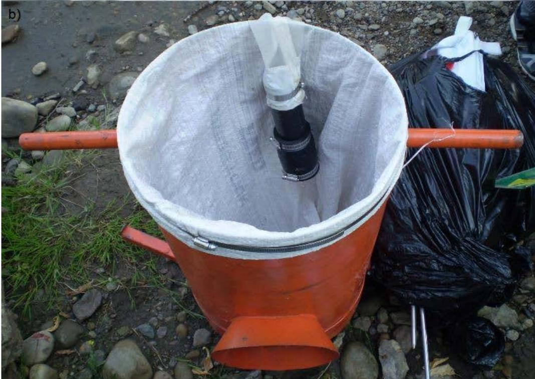
FIGURE 2-3 a) Front view of a Neill cylinder showing the grate, foot bars on the bottom of the sides and handlebars on the sides; b) Top view of a Neill cylinder showing the top opening with an attached covering, handlebars, and the drift net wrapped around into the top from the back with a clamp at the end for attaching a 1L nalgene bottle
