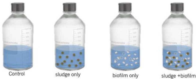
Figure C-4. Set up of the batch test bottles, each bottle was in triplicates.
