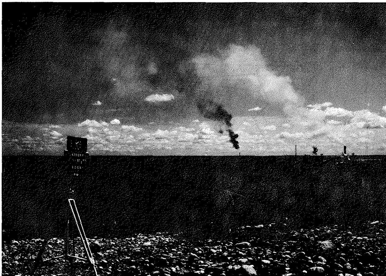
Figure 24. Photograph of looping GCOS plumes. The white plume is from the power plant stack; the dark plume is from the flare.
