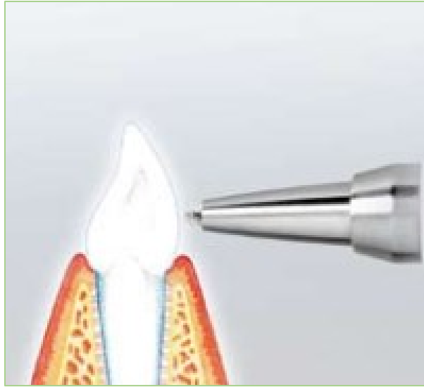
Figure 2.9: Periotest Mechanism Applying an Impact Load to Excite Vibration in a Tooth (from http://www.med-gulden.com/downloads/02_english/01_Productinformation/Periotest_procedure.pdf )
