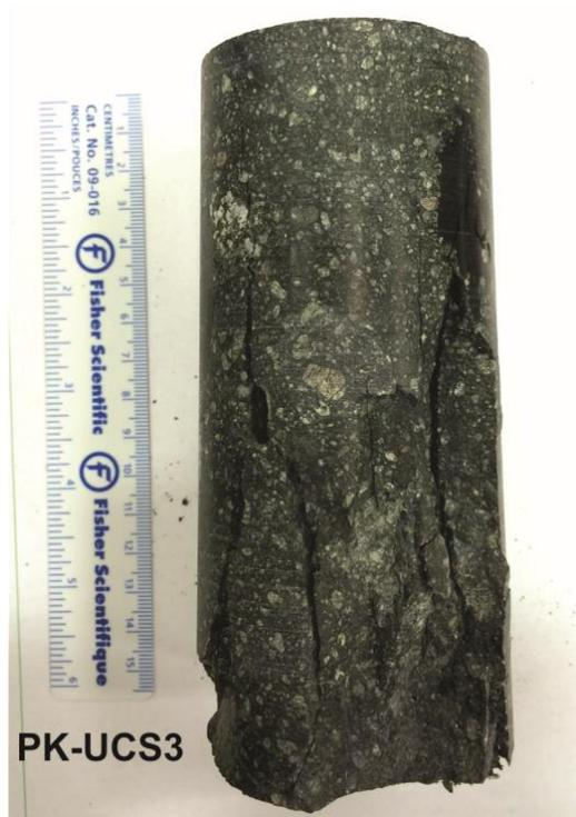
Figure 3.6 Example of mode of failure from a UCS test (Sample ID: PK-UCS3)
