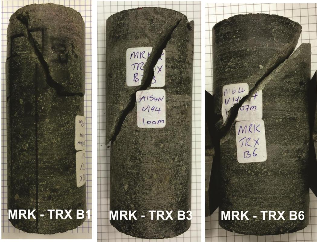
Figure A.58 Failure Mode of Each Core Specimen - MRK Kimberlite - Triaxial Test
