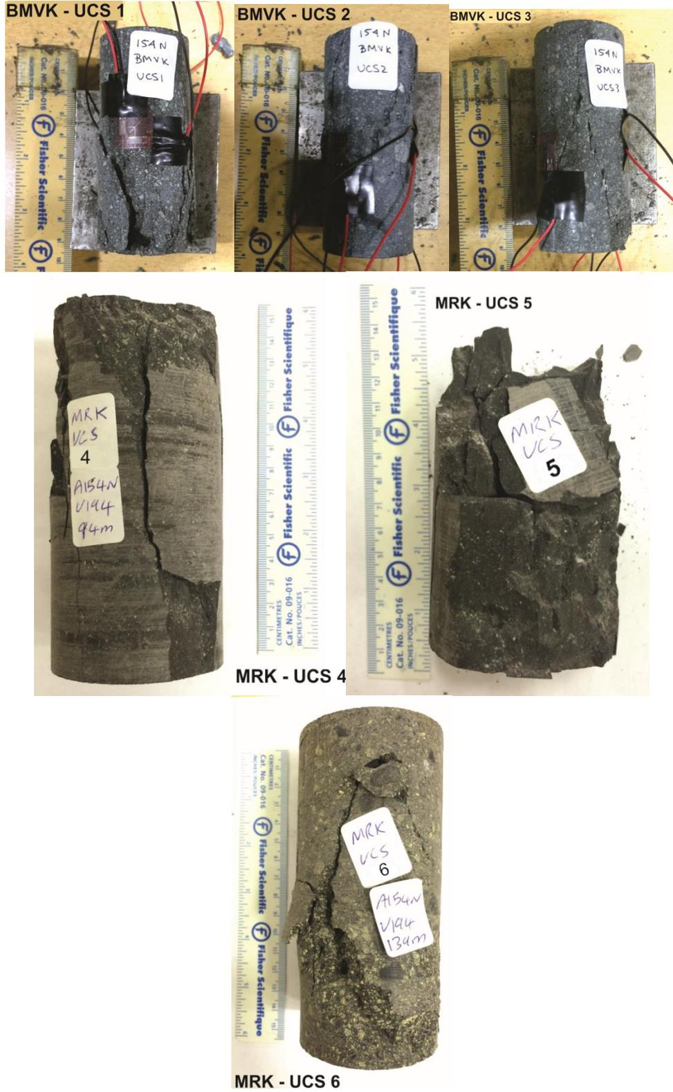
**Figure A-20** Uniaxial Compressive Strength Tests Results - Failure Modes for BMVK and MRK Rock Types
