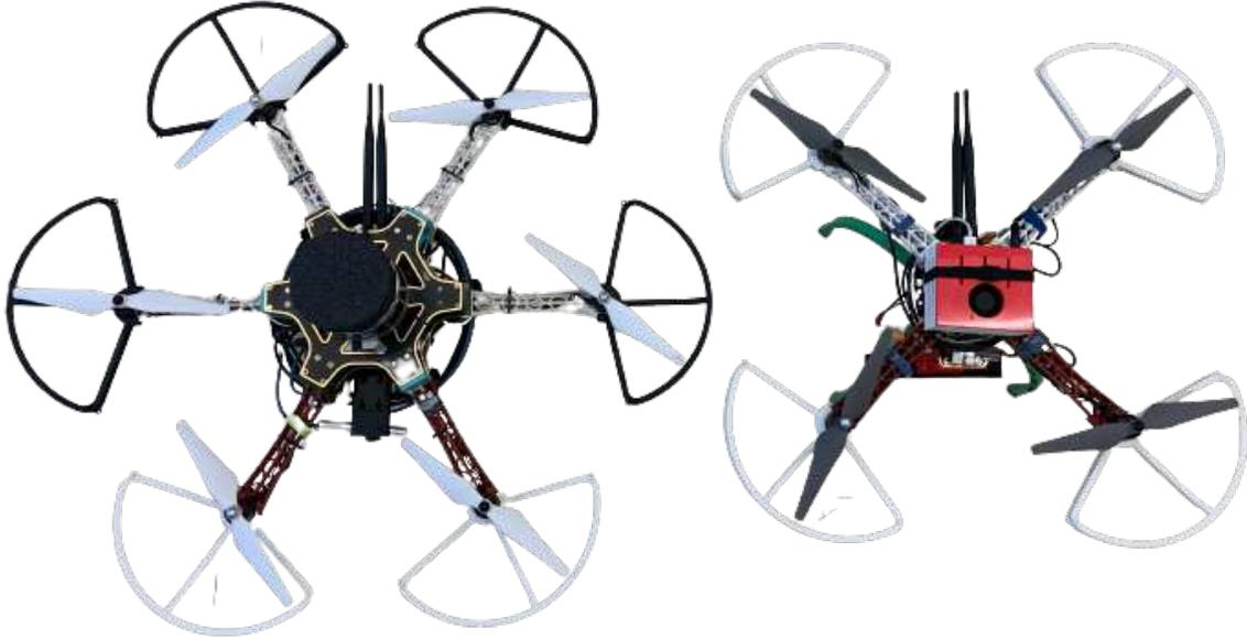
Figure 3.2: Top-view of prototype hexacopter (left) and quadcopter (right) designs.
