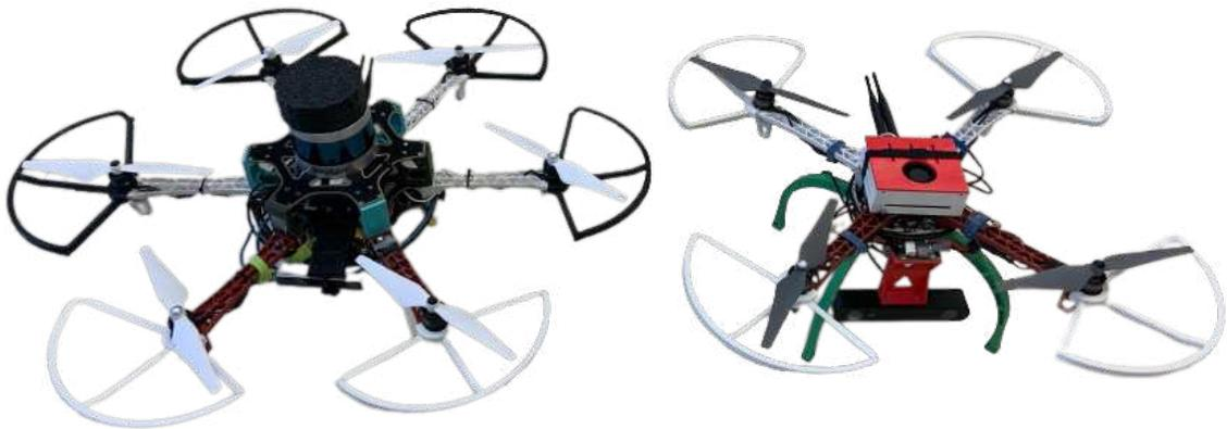
Figure 3.1: Side-view of prototype hexacopter (left) and quadcopter (right) designs.
