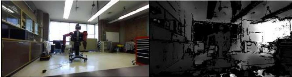
Figure 3.5: Standard and depth images produced by the ZED 2 camera.
