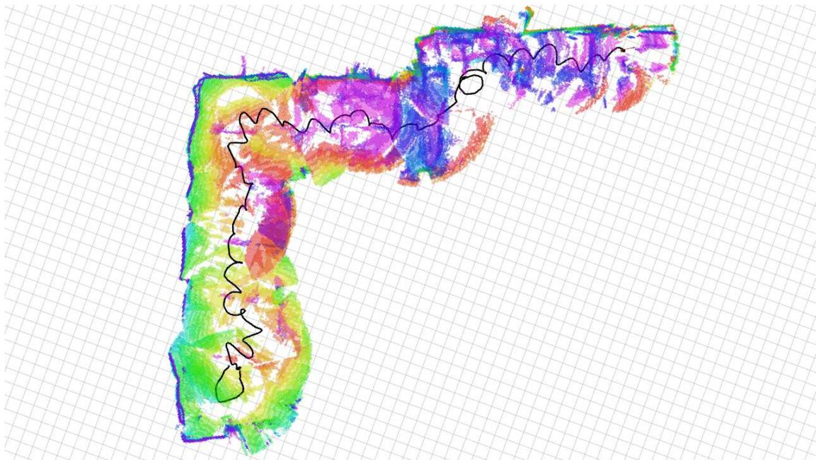
Figure 5.11: 3D perspective of the tracked trajectories by the quadcopter system in the underground space using the adapted exploration algorithm.
