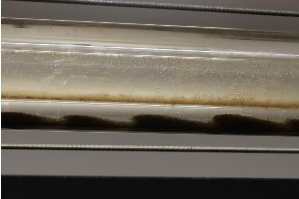
Figure 7-15 Typical Shape of Dunes for Experiments with Water and Fine Particles
