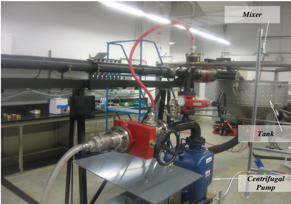
Figure 3-2 Pictures of the Flow Loop Component; The Tank, Pump, Mixer and Safety Valves and also Bypass line Could be Observed in the Picture
