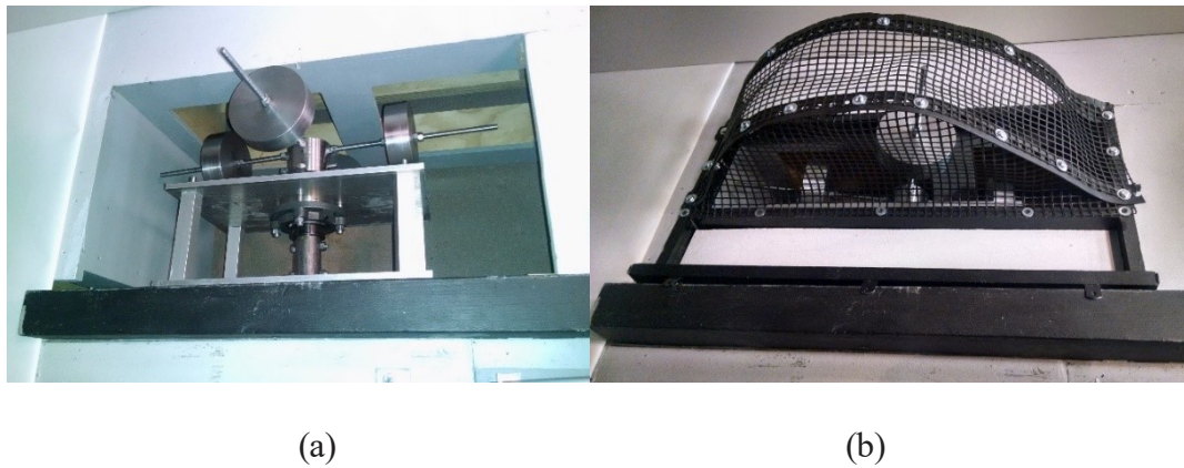
Figure 0-3 (a) The linear inertia system, exposed and without protection, (b) the mass guard placed on the linear inertia system
