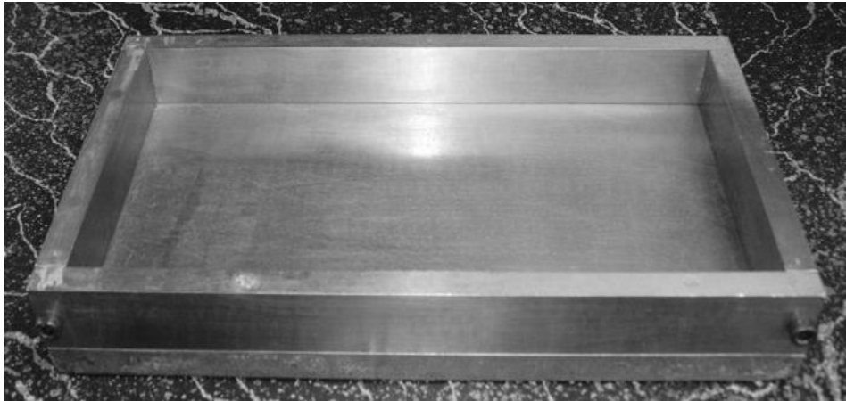
Figure 2.5 Mold used for epoxy casting.
