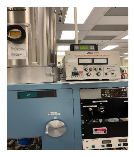
Figure 5: Electron Beam-Physical Vapor Deposition (EB-PVD) chamber at the UofA nanoFAB
