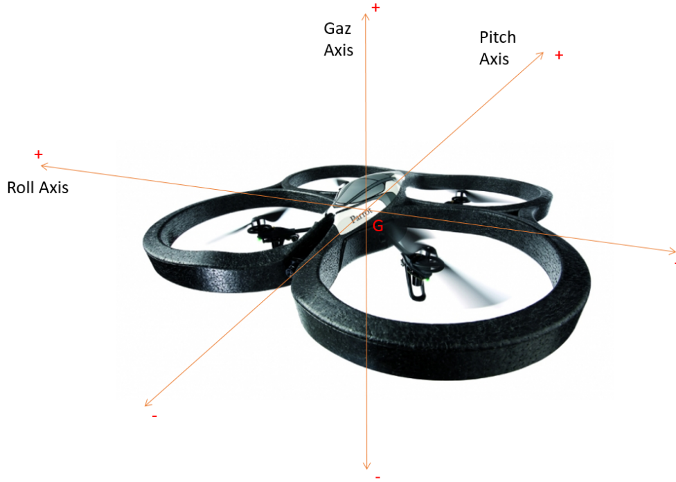
Figure 4.13: Parrot AR.Drone 2.0 Motion Axis Representation
