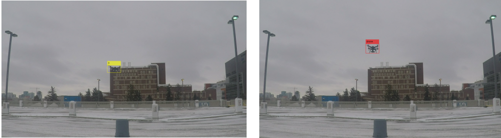
Figure 3.8: Blob Analysis Test with Static Camera: HOG-FAST Detection Process plus Hungarian Assignment Algorithm with Kalman Filter Tracking
