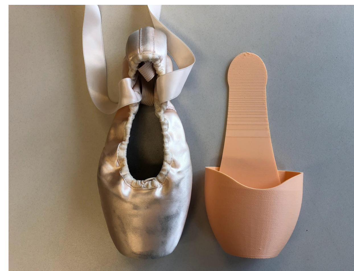
Fig. 4. Pointe shoe and 3D printed box and shank
