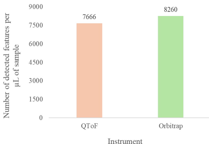
Figure 5.4. The number of detected features detected in QToF and Orbitrap normalized by the amount of raw samples injected ( i.e. , 2 \mu\text{L} for Orbitrap samples and 1.88 \mu\text{L} for QToF samples).
