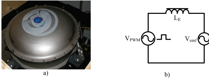
Fig. 1-4. Flywheel battery system: a) example photograph and b) simplified electrical model of a permanent magnet synchronous machine. ' V_{emf} ' is the back electromotive force of the electric machine, and ' V_{PWM} ' is the pulse-width modulated converter voltage.
