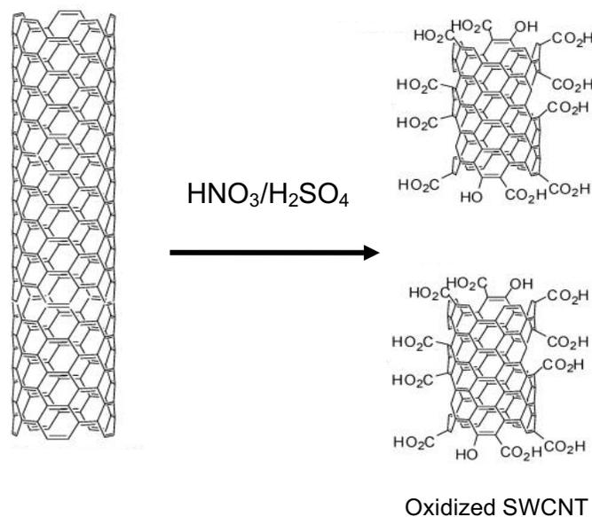
**Figure S5-1. Schematic of oxidation process used to purify and functionalize CNT-30, CNT-40 and CNT-50 from U-CNTs.** U-CNTs were produced by the induction thermal plasma process (Kim et al., 2007). U-CNTs were oxidized in a  $\text{HNO}_3/\text{H}_2\text{SO}_4$  mixture for 2 h at 30, 40, and 50 °C to yield mostly carboxylic acid groups on the ends and sidewalls, termed CNT-30, CNT-40 and CNT-50 respectively.
