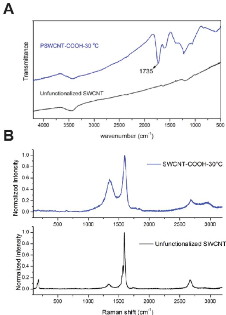
**Figure S3-2. Infrared and Raman spectroscopy verified the introduction of carboxylic acid group functionalization to CNT-30.**
