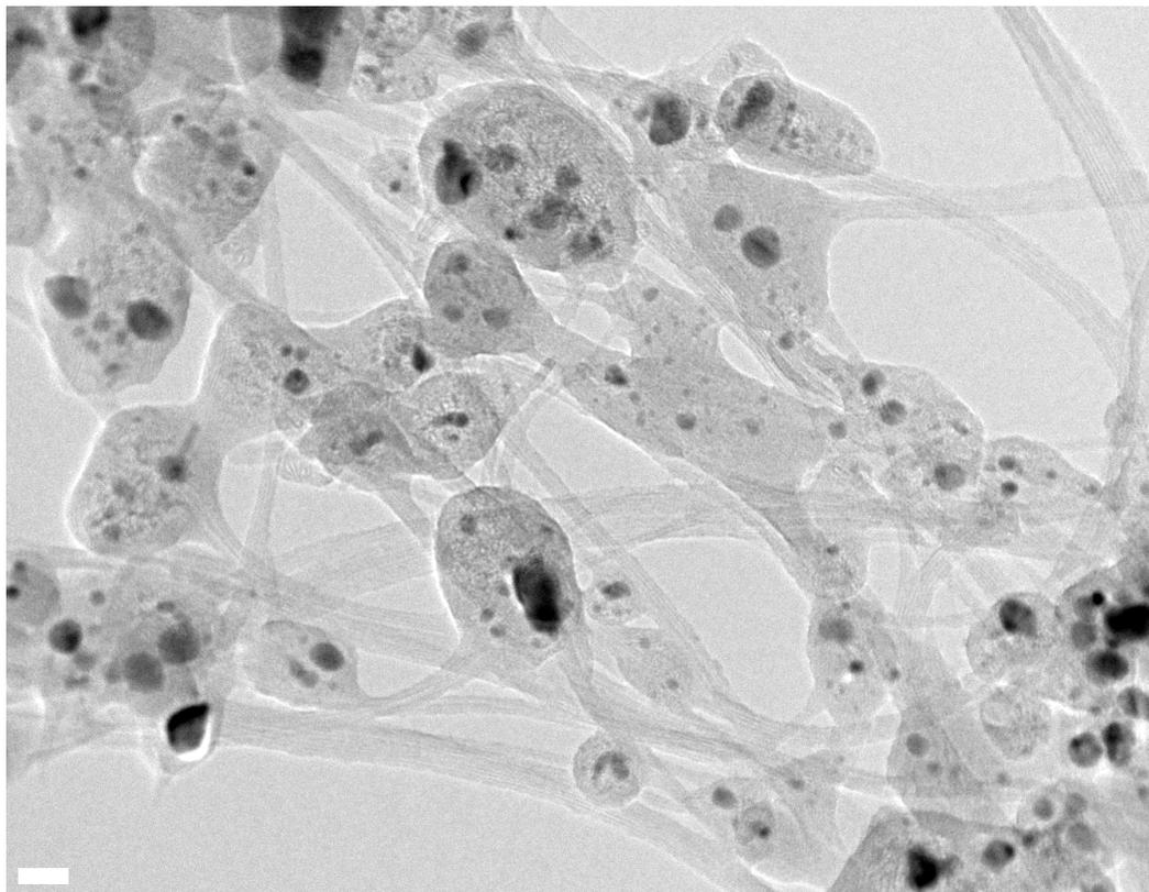
**Figure S3-1. Unfunctionalized CNTs (U-CNTs) have a diameter of ~1.5-1.6 nm and extend in parallel bundles up to several micrometers in length.** High resolution transmission electron microscopy micrographs of U-CNTs produced by induction thermal plasma technique before purification and oxidation. Scale bar = 20nm.
