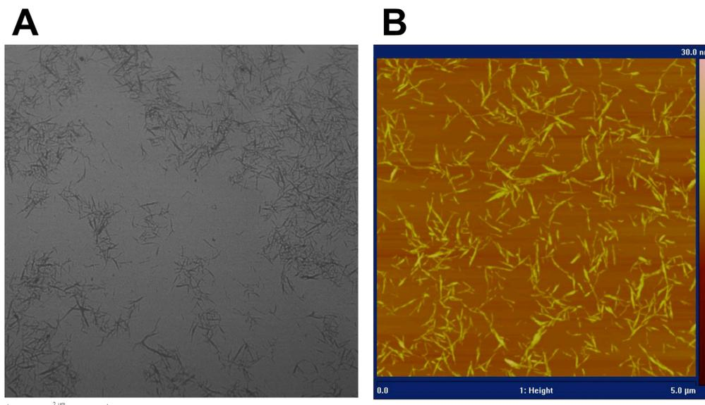
**Figure S6-1. Low voltage transmission electron microscopy (LVTEM) micrographs (A) and height mode atomic force microscopy (AFM) micrographs (B) of crystalline nanocellulose (CNC) produced using the APS method. CNCs were uniform in size, with an average length of  $128 \pm 4$  nm and diameter of  $5.5 \pm 0.1$  nm.**
