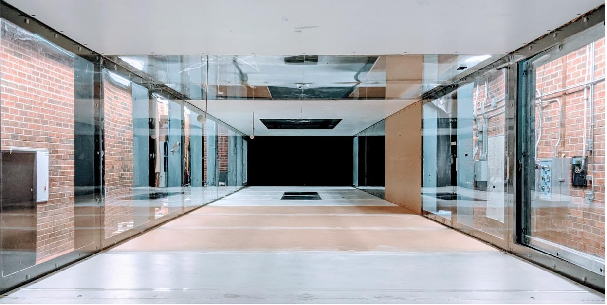
Figure 3.1: The test section of the wind tunnel in the Mechanical Engineering Building at the University of Alberta.
