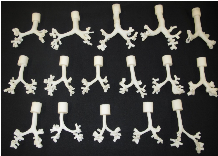
Figure 2.2: 5 anatomically realistic adult hollow tracheobronchial replicas (top row) and 11 anatomically accurate child hollow tracheobronchial replicas (second and third rows)
