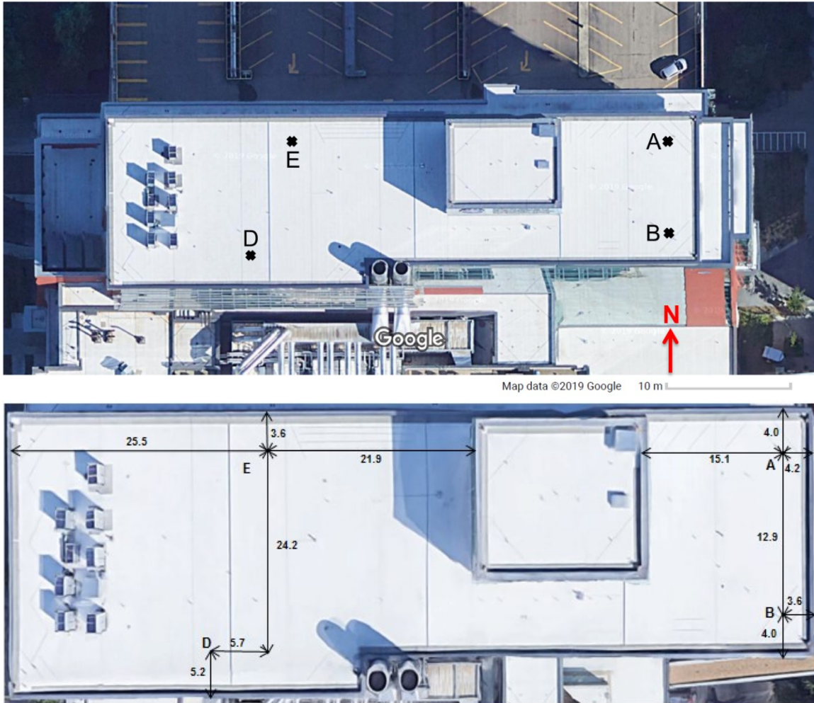
Figure 3-6: Locations of anemometers on the roof of the DICE building (not to scale). Note that dimensions are in m.
