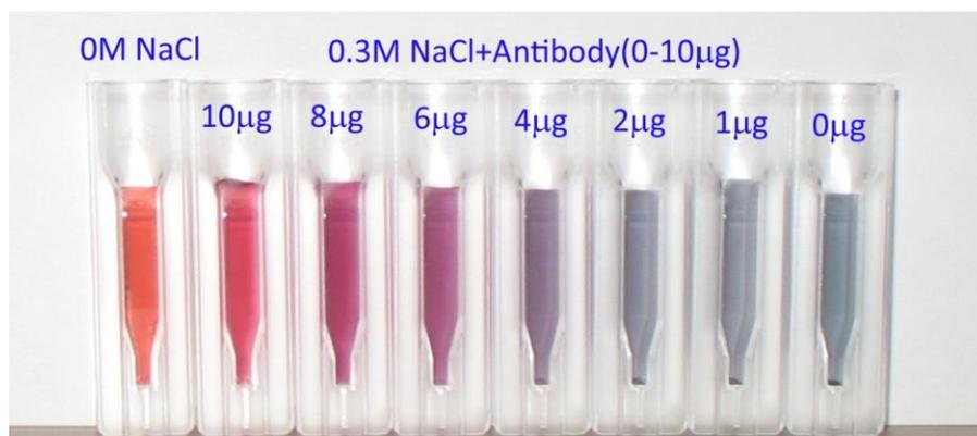
**Figure 2.** Result of antibody loading test. The far left tube contains Au NPs in water with no salt or antibody added. To the other tubes containing the same amount of Au NPs was added varying amounts (0–10 µg) of antibody and 1 M NaCl.
